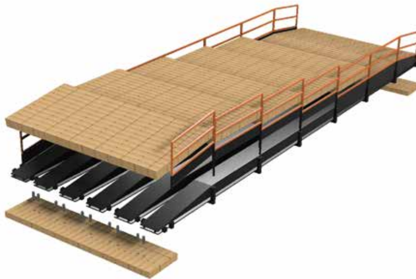
Expanded view of Sterling's TerraCross 56 bridge system including beam assemblies, bearing mats, decking mats, and handrails. Other TerraCross bridges may include different components.
